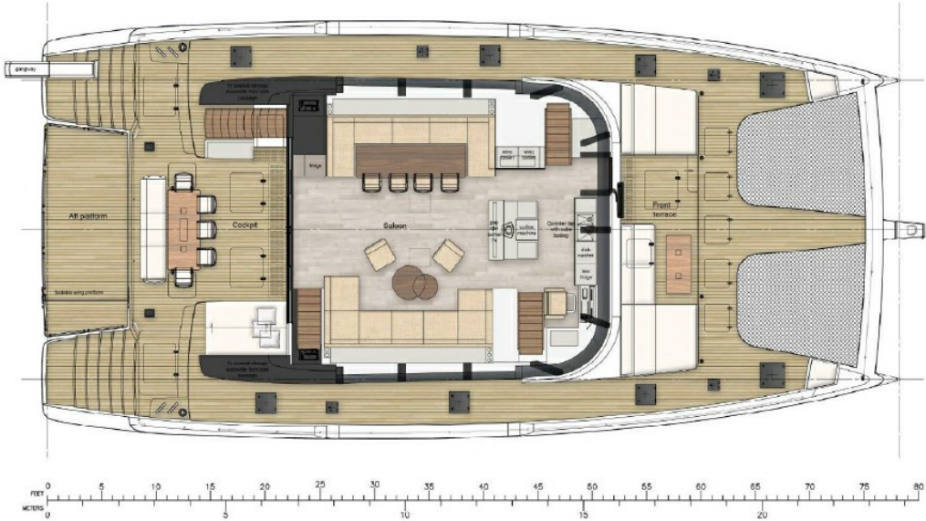
General Arrangement - Main Deck
